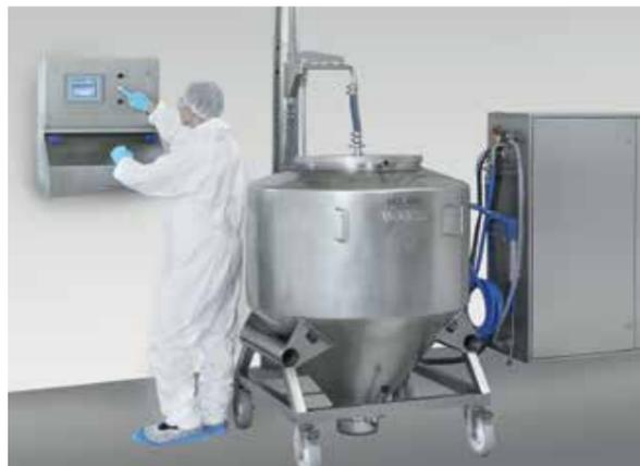
All of the components for transporting and treating the cleaning water are stored within a compact stainless steel cabinet. Washing processes are performed on the basis of recipes and are automatically logged. A touch panel on the device enables convenient local operation.
